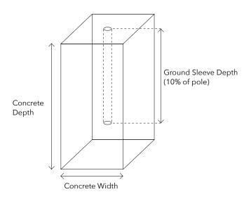
**NB:** We recommend that the concrete used in the bases should be of a C30 quality as normally purchased from a ready mixed concrete supplier. If purchaser is to mix concrete up themselves then the ratio of the mix i.e. Cement/Sand/Fine Aggregate must 1:2:3 which results in a very strong mix. Any deviation from the above advise may result in warranty claims being invalid. If in any doubt please contact supplier for clarification.
